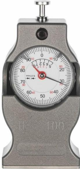
Zero setter for smaller tools. Use with smaller drills and mills
